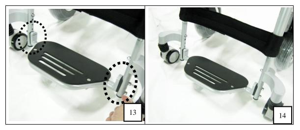
• After loosening the screws the Footrest height can be adjusted using the different holes at 1.8cm distance.
