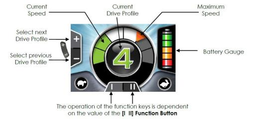
The colour of the current Drive Profile, shown in the middle of the screen, is dependent on the chair's status.
