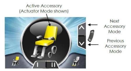
When the Accessory Mode button is pressed (either Next or Previous) the menu will always start at the Seating Accessory screen (if actuators are active).
